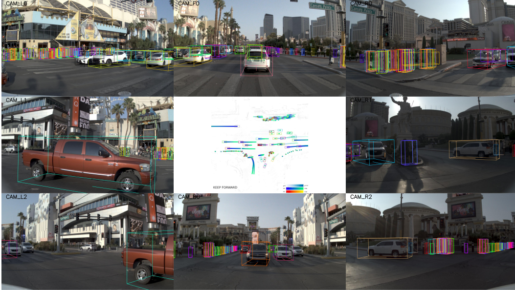
Figure 2: Visualization of the PARA-Drive Model’s output. Eight surrounding cameras are displayed with detected object bounding boxes. In the center, the predicted BEV information is shown, including object bounding boxes, their predicted multi-modal future trajectories, as well as the planned trajectory for the ego vehicle.
